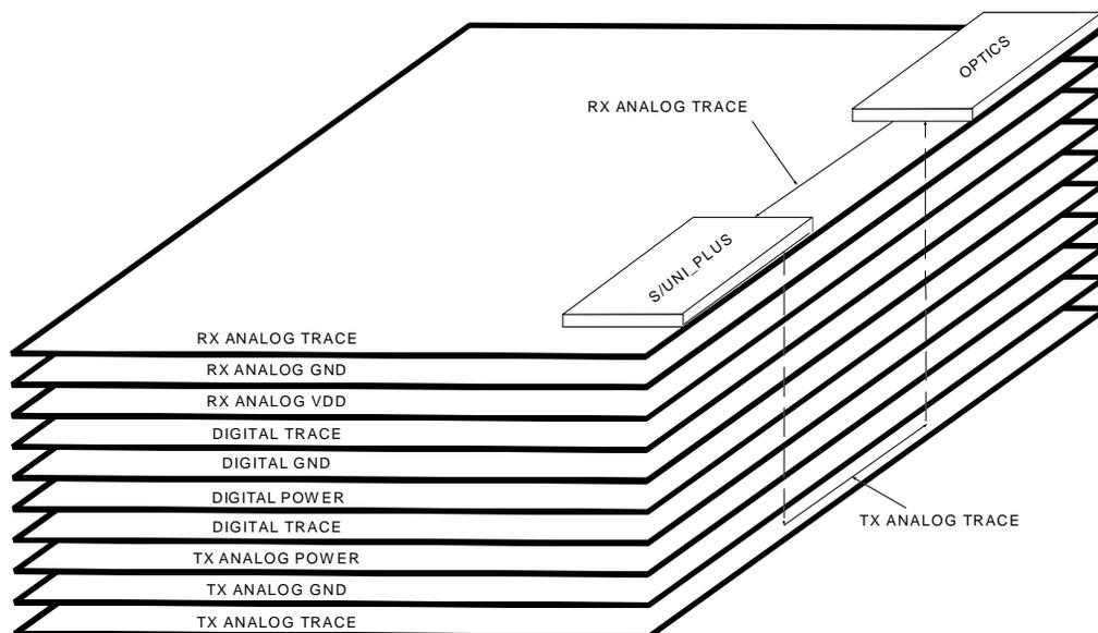
**Figure 3: Recommended Power/Ground Plane Connection on a Ten Layer Board**
