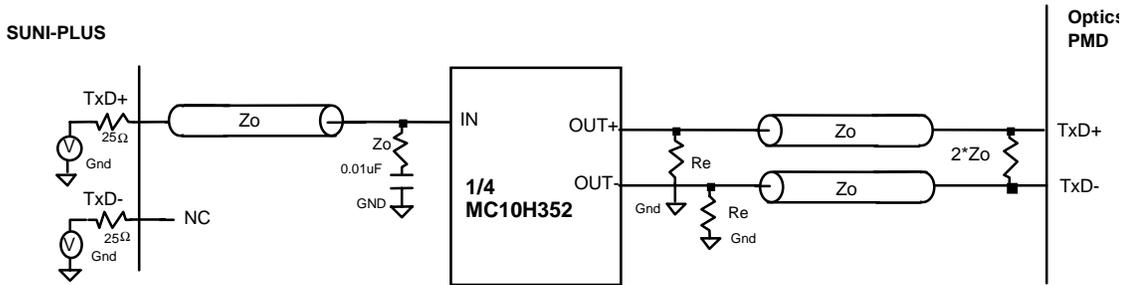
The value of  $R_e$  is dependent on the signal trace characteristic impedance and the ECL or PECL supply voltage (-4.5 V, + 5 V). Values in the range of 330  $\Omega$  are recommended
