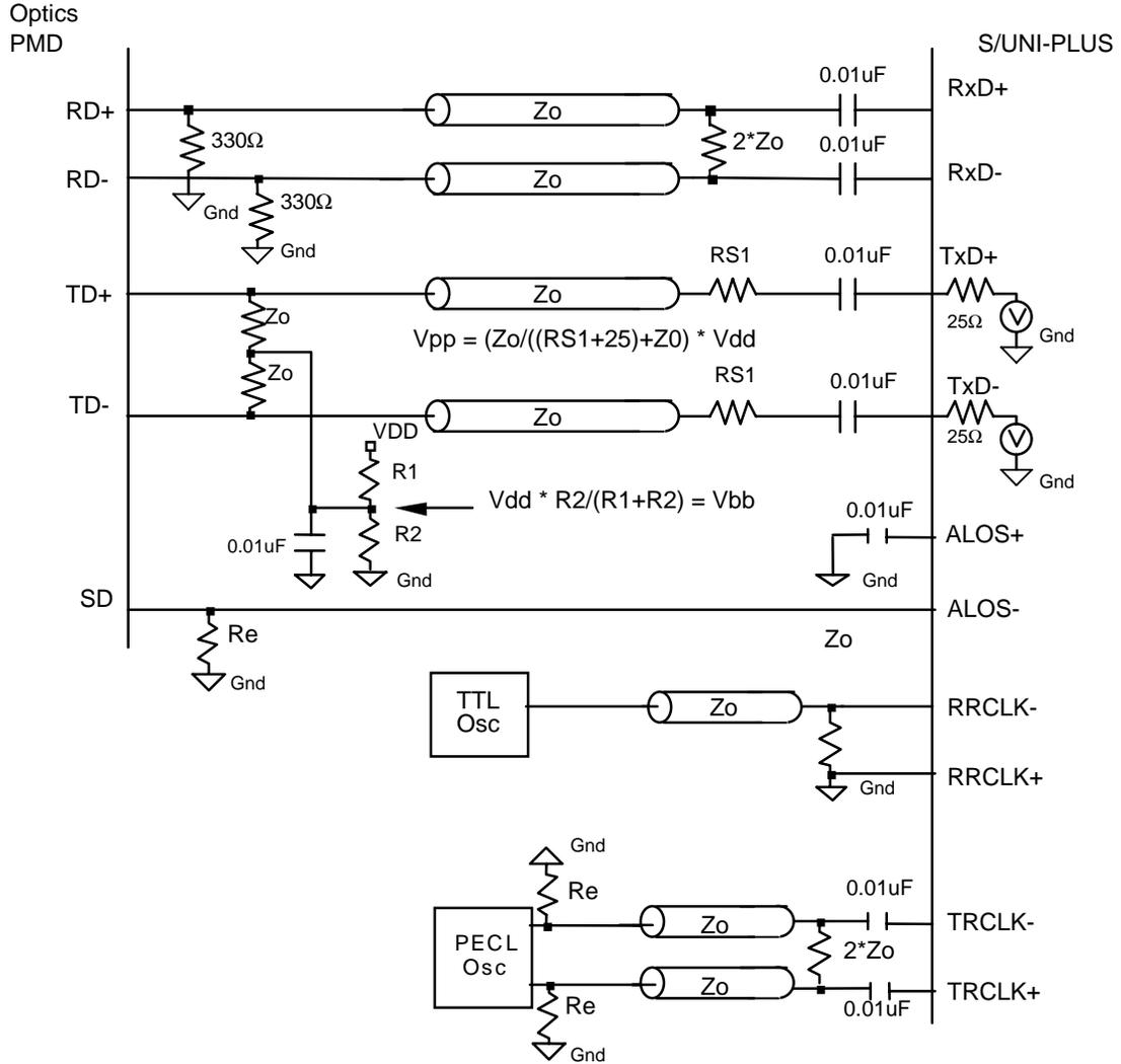
Notes:  $V_{pp}$  is minimum input swing required by the optical PMD device.
