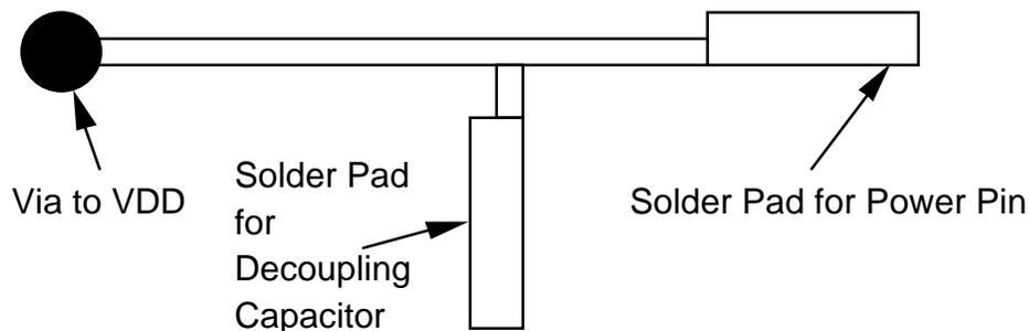
**Fig. 1: Recommended Layout for VDD Decoupling Connection to Analog Power Pins**
