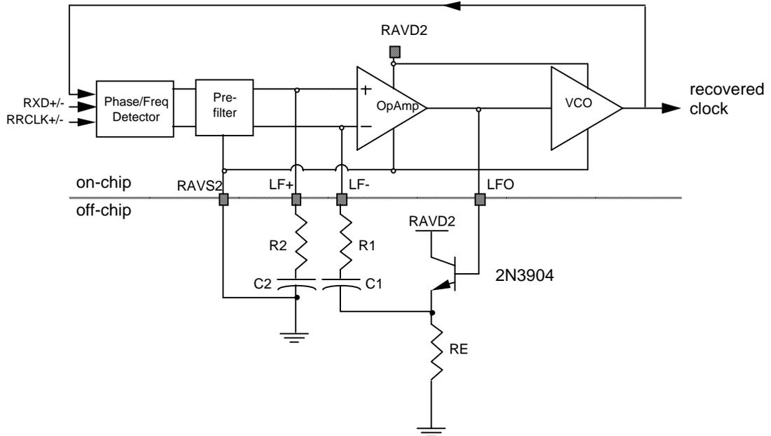
The capacitor values are the minimum recommended values; larger values of capacitance can be used on any of the line rates without affecting performance of the SUNI-PLUS.
