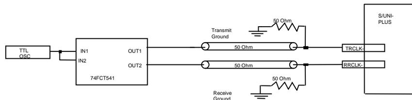
The TTL oscillator should be placed as close to the buffer as possible as it is unterminated. The TTL oscillator is used to match the 74FCT541's TTL input level in order to avoid duty cycle distortion caused by differences in output levels and input switching thresholds.
