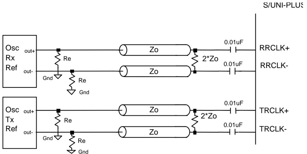
The value of  $R_e$  is dependent on the signal trace characteristic impedance and the ECL or PECL supply voltage (-4.5 V, + 5 V). Values in the range of 200-330  $\Omega$  are recommended
