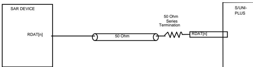
A modified version of this termination scheme must be used when a multi-phy SAR bus is connected to more than one S/UNI-PLUS. This is shown in the next diagram.
