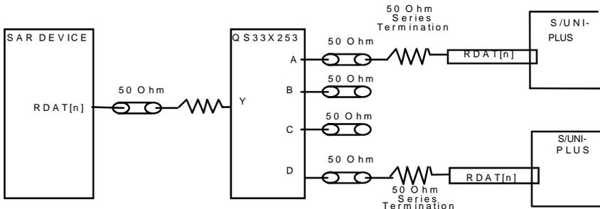
The QS33X253 acts like a 4-1 multiplexer and each interconnect can be thought of as a single point to point connection terminated by a series resistor.
