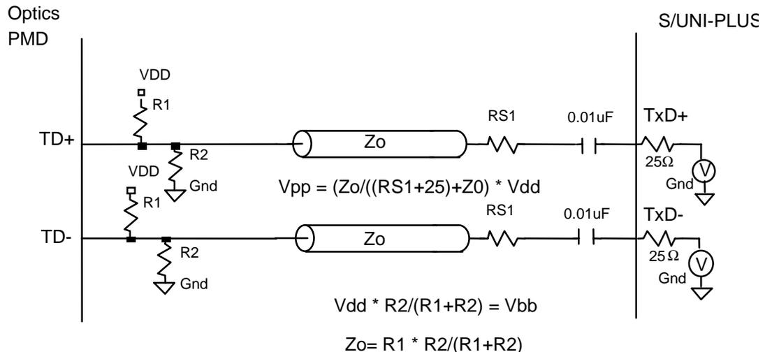
Notes:  $V_{pp}$  is minimum input swing required by the optical PMD device.
