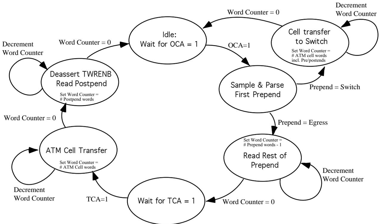
**Fig. A5 Block Diagram of the Egress Routing Glue Logic**
