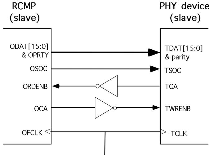
**Fig. 6 Slave-slave interface timing**
