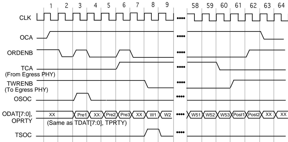
Fig. A3 shows the timing diagram of a typical Egress cell transfer for an 8-bit interface. The following describes the sequence of events for the transfer of a cell with 3 prepend words (the first one for Egress routing) and 2 postpend words.
