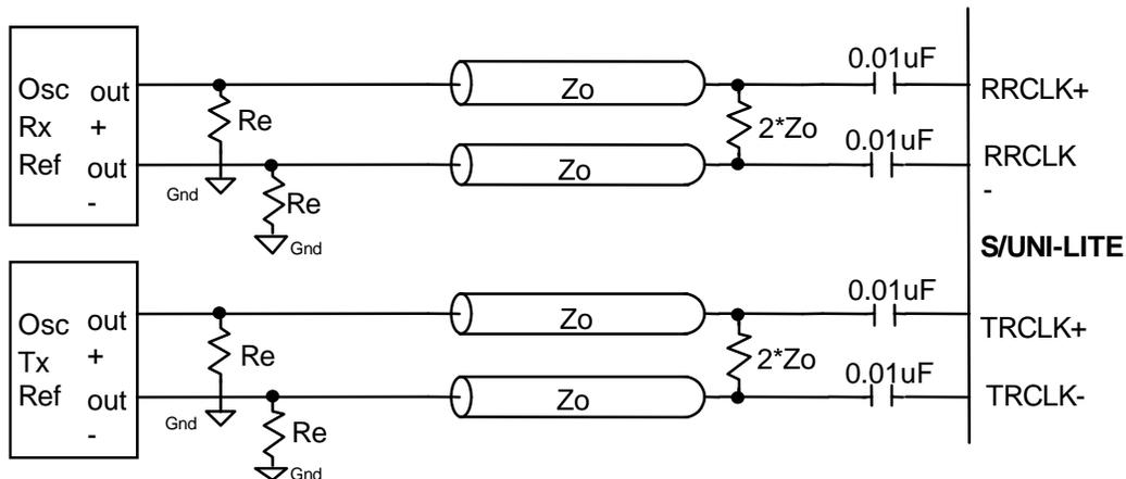
The value of  $R_e$  is dependent on the signal trace characteristic impedance and the ECL or PECL supply voltage (-4.5 V, + 5 V). Values in the range of 200-330  $\Omega$  are recommended
