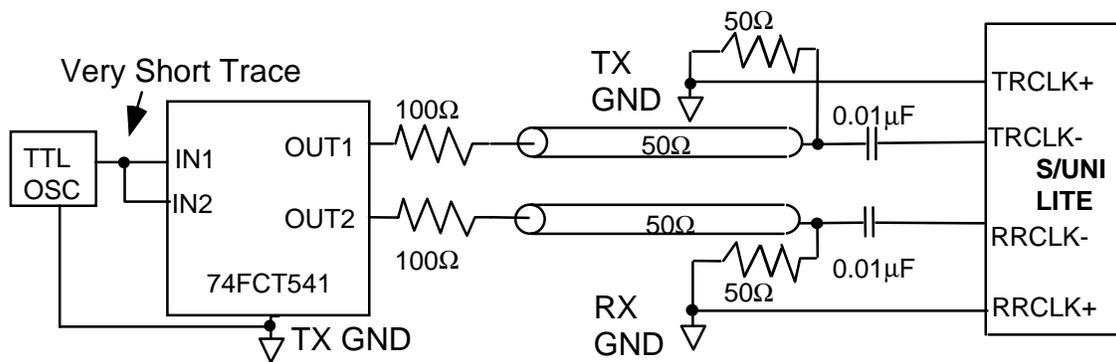
The TTL oscillator should be placed as close to the buffer as possible as it is unterminated. The TTL oscillator is used to match the 74FCT541's TTL input level in order to avoid duty cycle distortion caused by differences in output levels and input switching thresholds.
