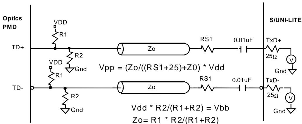
Notes: V<sub>pp</sub> is minimum input swing required by the optical PMD device.
