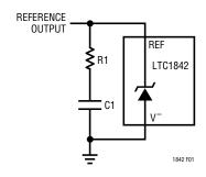
Figure 1. Damping the Reference Output
