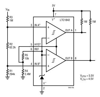
Figure 5. Dual Level Detector
