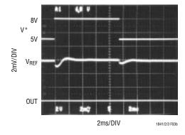
Figure 3b. Power Supply Transient Rejection
