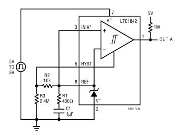
Figure 3a. Power Supply Transient Test Circuit
