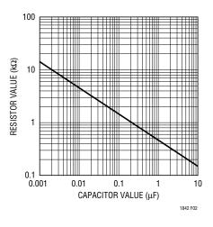
Figure 2. Damping Resistance vs Bypass Capacitor Value
