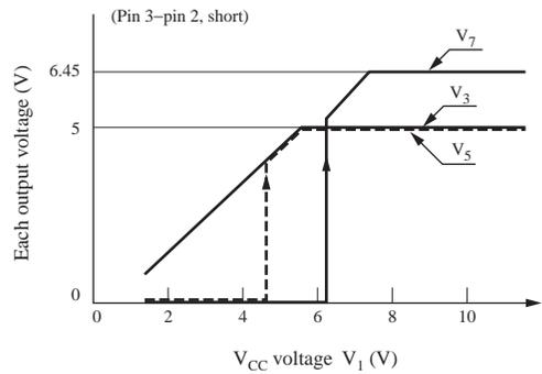
3) Timing relationship of regulator output voltage vs. reset output
