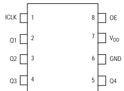
**Figure 2. Pin Assignment**
