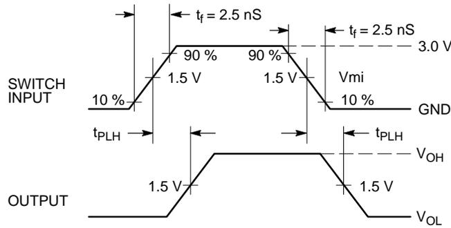
**Figure 5. Propagation Delays**
