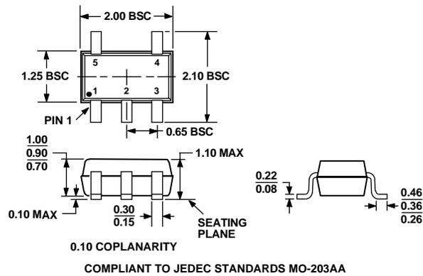
Figure 21. 5-Lead Thin Shrink Small Outline Transistor Package [SC70] (KS-5)
