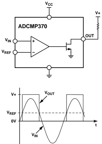
Figure 18. Basic Comparator and Input and Output Signals
