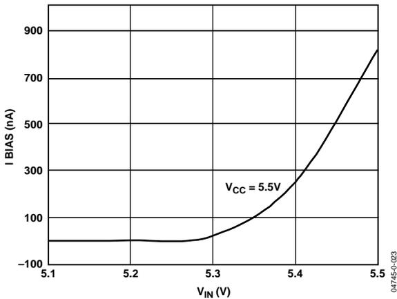
Figure 13. Input Bias Current vs. Input Voltage
