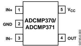
Figure 3. Pin Configuration
