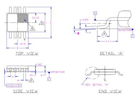
Figure 1 8-Pin TSSOP Package Outline - 3x3mm Body 0.65mm Pitch
