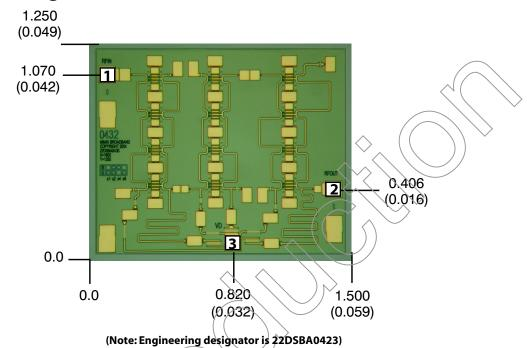
Units: millimeters (inches) Bond pad dimensions are shown to center of bond pad.
