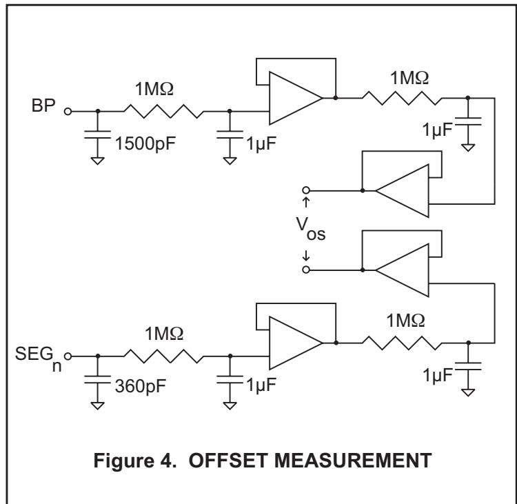
**Figure 4. OFFSET MEASUREMENT**
