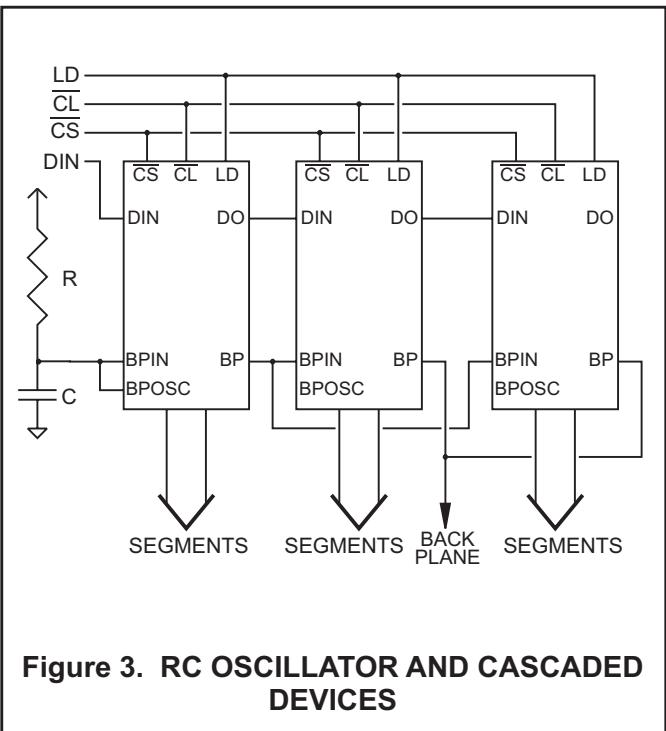
**Figure 3. RC OSCILLATOR AND CASCADED DEVICES**
