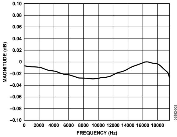
Figure 3. ADC Pass-Band Filter Response, 48 kHz
