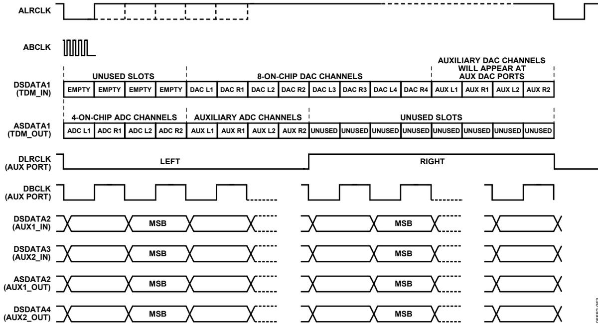
Figure 17. Combined AUX DAC and ADC Mode
