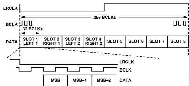
Figure 12. ADC TDM (8-Channel I<sup>2</sup>S Mode)
