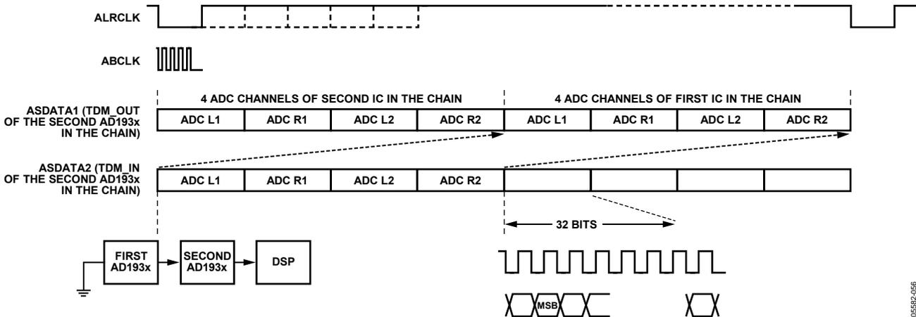
Figure 21. ADC TDM Daisy-Chain Mode (256 f<sub>s</sub> BCLK, Two AD1938 Daisy Chain)
