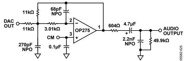
Figure 32. Typical DAC Output Filter Circuit (Single-Ended, Inverting)
