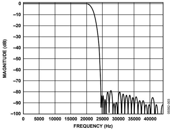
Figure 4. ADC Stop-Band Filter Response, 48 kHz
