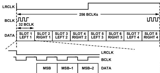
Figure 13. DAC TDM (8-Channel I<sup>2</sup>S Mode)
