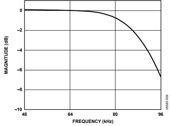
Figure 10. DAC Stop-Band Filter Response, 192 kHz
