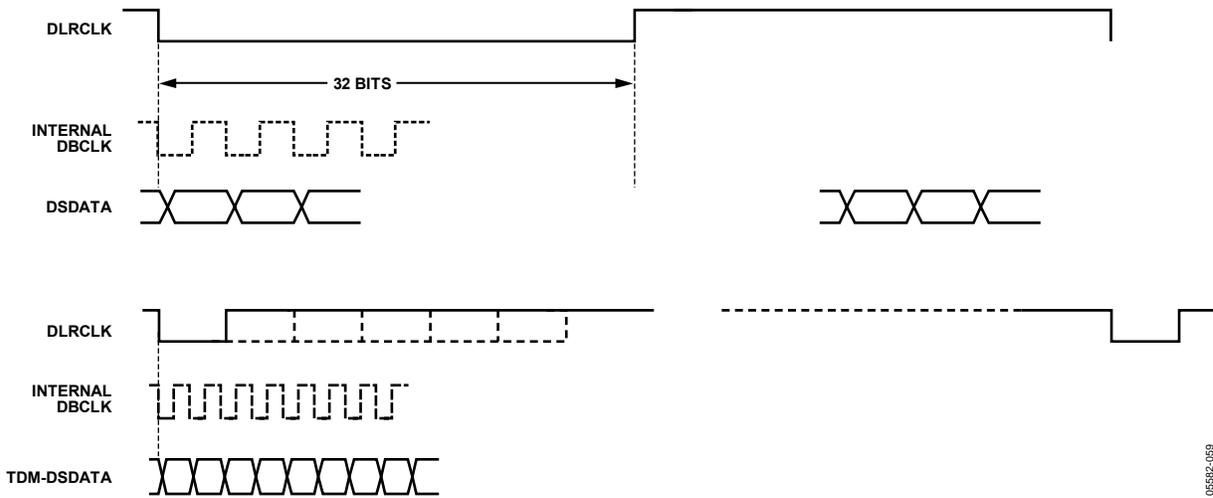
Figure 27. Serial DAC Data Transmission in TDM Format Without DBCLK
