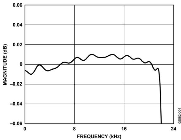
Figure 5. DAC Pass-Band Filter Response, 48 kHz
