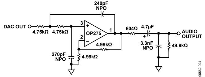
Figure 31. Typical DAC Output Filter Circuit (Single-Ended, Noninverting)
