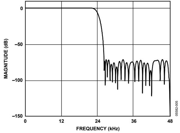
Figure 6. DAC Stop-Band Filter Response, 48 kHz
