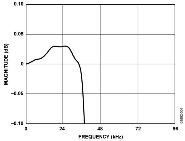
Figure 7. DAC Pass-Band Filter Response, 96 kHz
