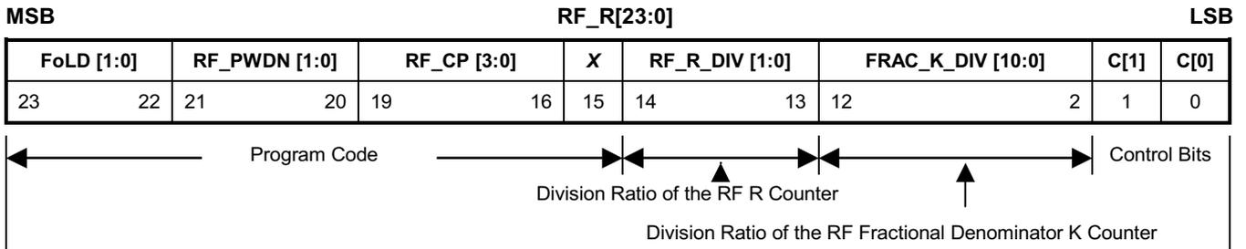
**Table.7 Binary 11-Bit Programmable Fractional Denominator K Divider Ratio (K Counter) (RF\_R[12:2])**
