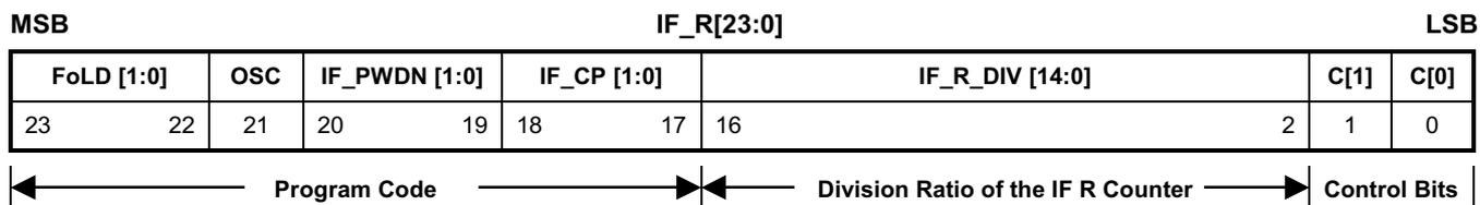
**Table.3 Binary 15-Bit Programmable IF R Divider Ratio (R Counter) (IF\_R[16] –IF\_R[2])**
