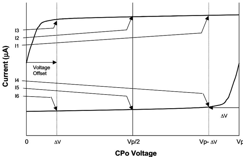
I1 = CP sink current at  $V_{CPo} = V_p - \Delta V$
