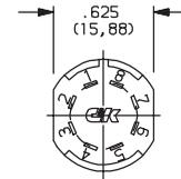
Terminal numbers molded on bottom of housing.
