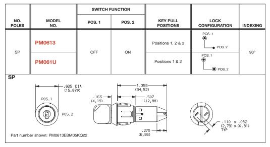
All models  ${}_{\circ}$   ${\bf M}$   ${\bf G}^{\circ}$   ${\bf M}$  with all options when ordered with 'Q' contact material.
