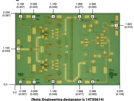
Units: millimeters (inches) Bond pad dimensions are shown to center of bond pad.
