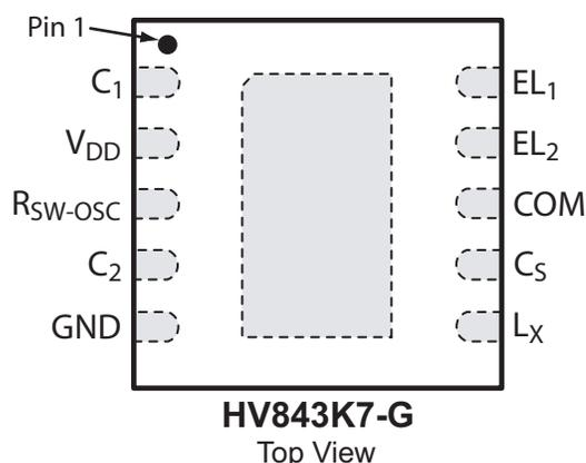
Note: Pads are on the bottom of the package.
