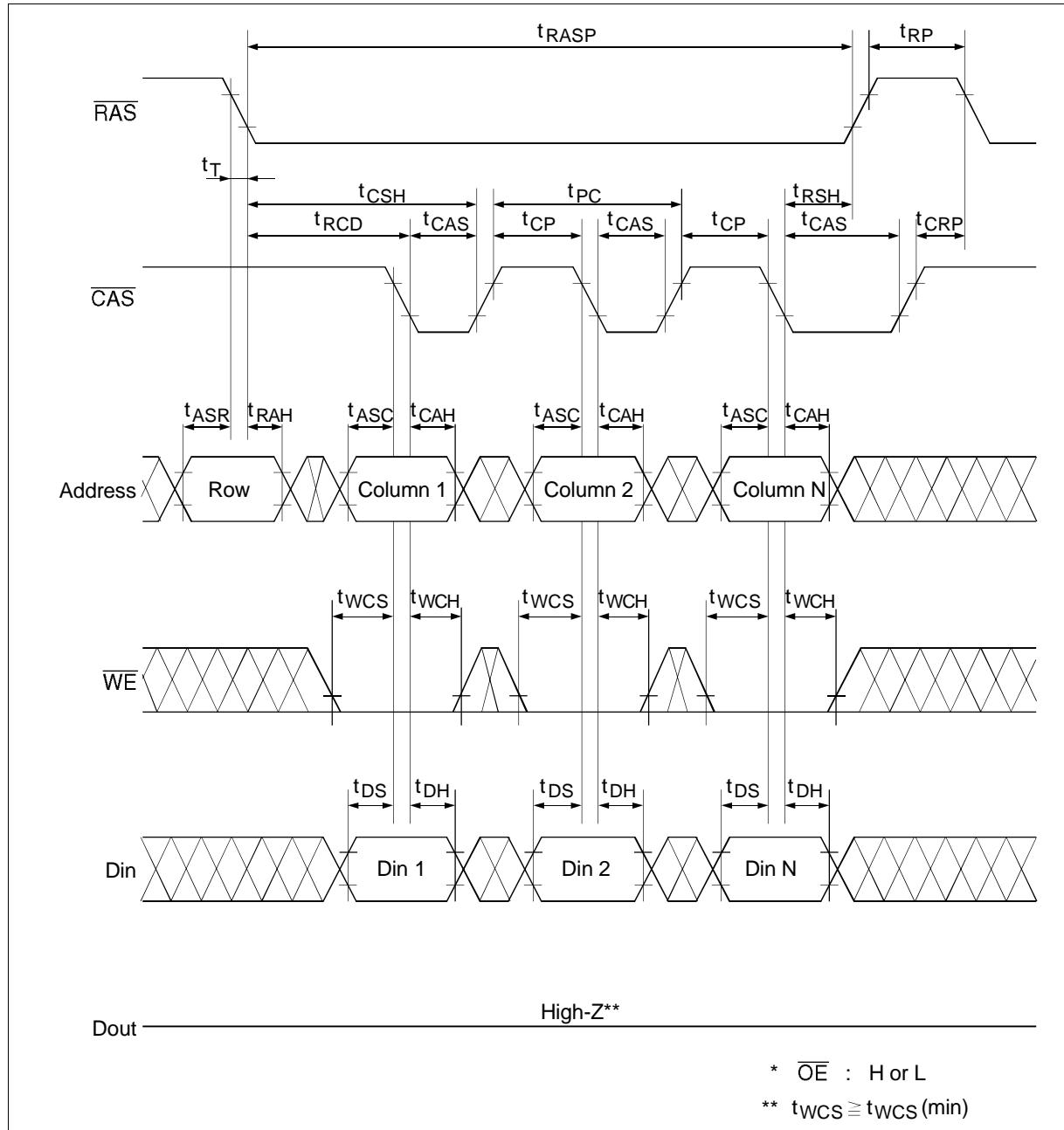
**Fast Page Mode Delayed Write Cycle \*<sup>18</sup>**
