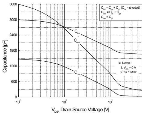
Figure 5. Capacitance Characteristics
