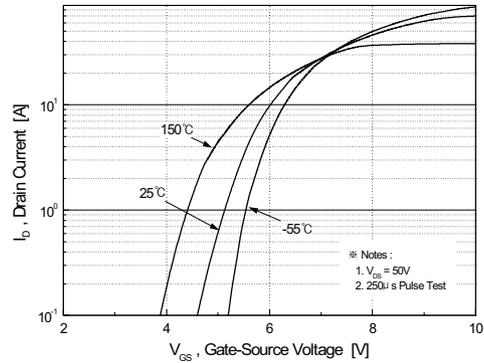
Figure 2. Transfer Characteristics
