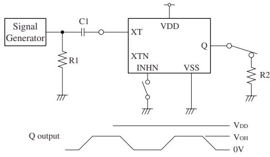
2Vp-p, 10MHz sine wave input signal
