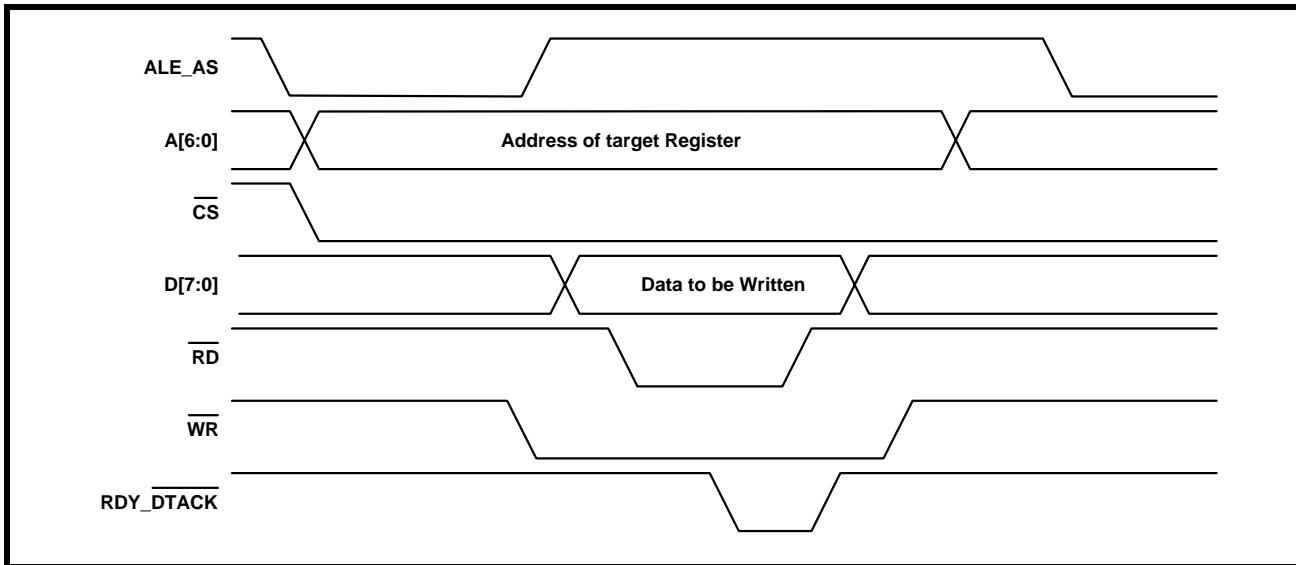
FIGURE 7. MOTOROLA \mu P INTERFACE SIGNAL DURING PROGRAMMED I/O WRITE OPERATION
