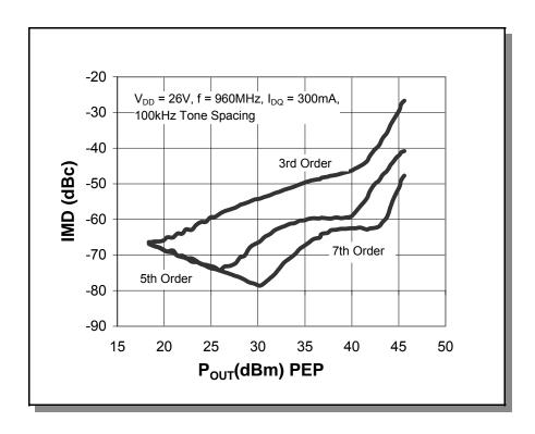
**Graph 2. Intermodulation Distortion vs. Output Power**
