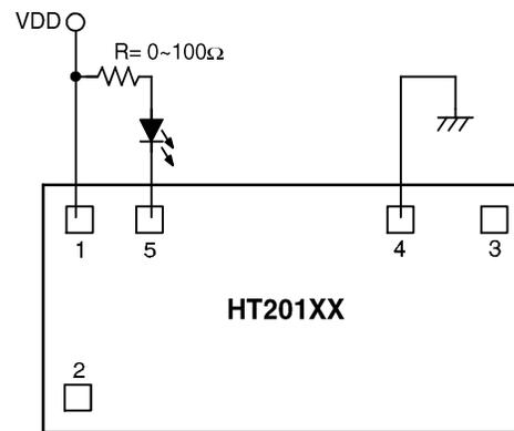
\*The IC substrate should be connected to VDD in PCB layout artwork.
