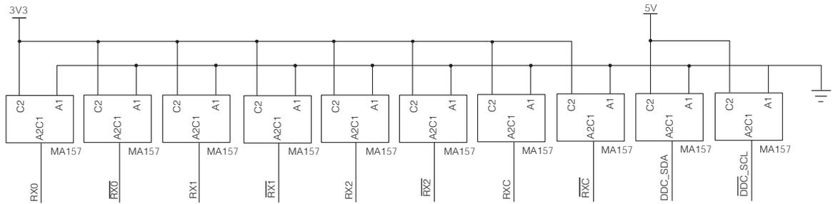
Note: For the DDC link to be active when the device is powered down, the 5V power to the DDC ESD diodes must be supplied by the DVI transmitter.
