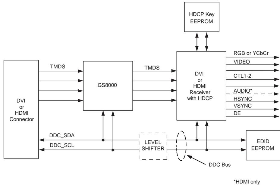
**Figure 3-2: LONG REACH™ DVI or HDMI Receive Solution**
