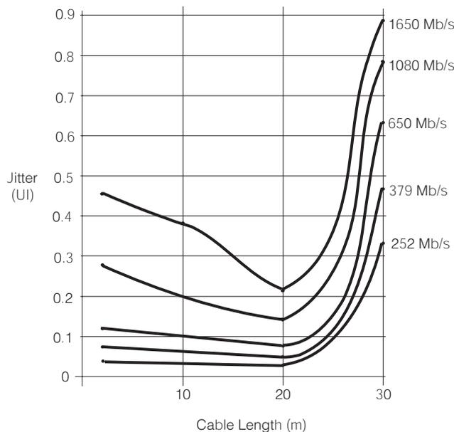
**Figure 2-1: Typical Additive Jitter vs. Cable Length**
