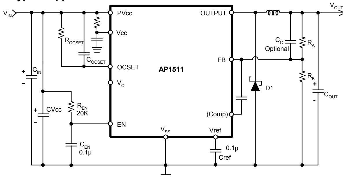
Note:  $V_{OUT} = V_{ref} \times (1 + R_A/R_B)$
