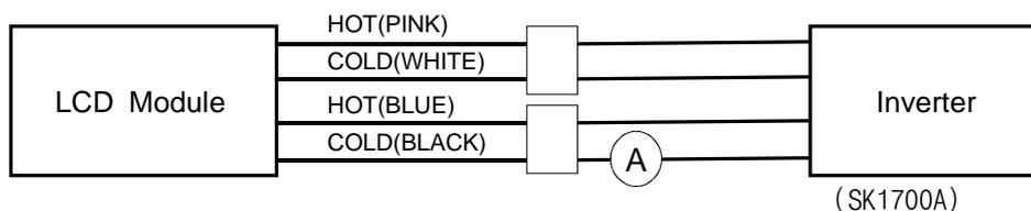
(2) Lamp frequency may produce interference with horizontal synchronous frequency and this may cause line flow on the display. Therefore lamp frequency shall be detached from the horizontal synchronous frequency and its harmonics as far as possible in order to avoid interference.
