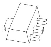
PBSS4250X 50 V, 2 A NPN low V<sub>CEsat</sub> (BISS) transistor
