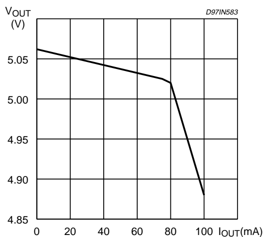
Figure 20: REG5 Regulator Characteristic (Vin = 6V, RUN3 = RUN5 = LOW, Tj = 25°C)
