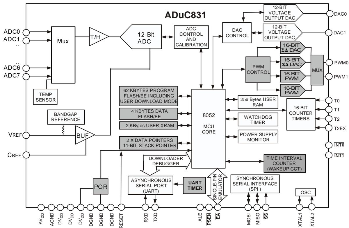
Figure 1 ADuC831 Block Diagram (Shaded areas are features not present on the ADuC812)
