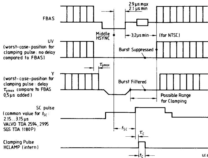
Leading edge at clamping pulse
