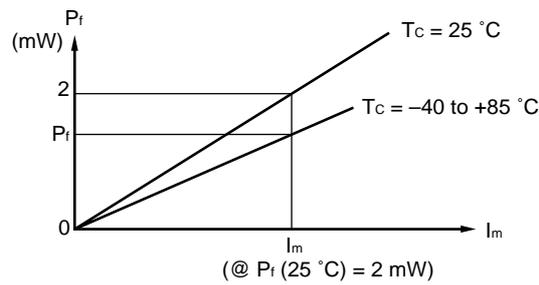
★ TYPICAL CHARACTERISTICS ( $T_c = 25\text{ }^\circ\text{C}$ , unless otherwise specified)
