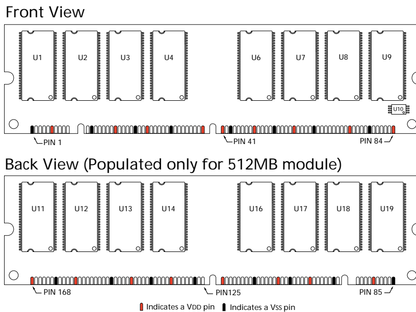
Figure 2: PIN Locations (168-PIN DIMM)
