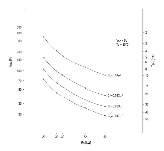
f<sub>FRM</sub> and T<sub>SCN</sub> vs. R<sub>0</sub> vs. C<sub>0</sub>
