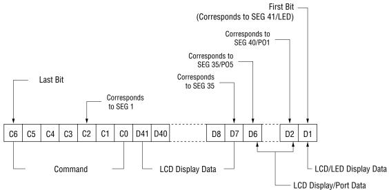
Notes: 1. LED data when the LED pin is selected and output port data when an output port pin is selected, correspond to common 1 side (C0, C1=0).
