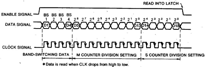
(2) When the control method selection pin SW is set to GND, the division ratio of the programmable divider and the band-switching output is as shown below.
