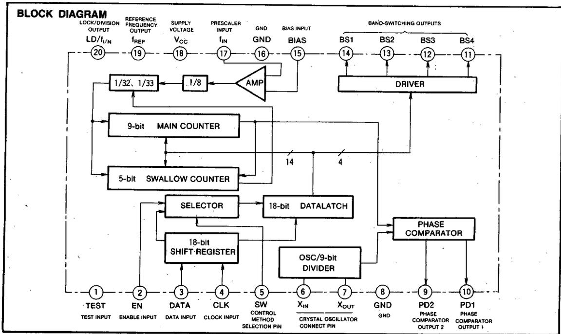
SERIAL INPUT PLL FREQUENCY SYNTHESIZER FOR VCR
