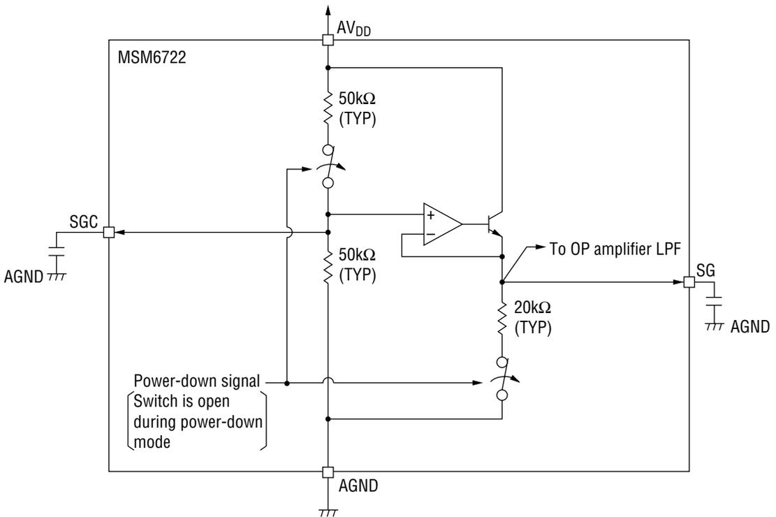
The SG signal is reference voltage (signal ground) for internal OP amplifiers and LPF. Install a capacitor between the SGC pin and AGND and between the SG pin and AGND respectively in order to make the SG signal noiseless. It is recommended to install an approx. 1μ capacitor, which should be determined after evaluating the tone quality.
