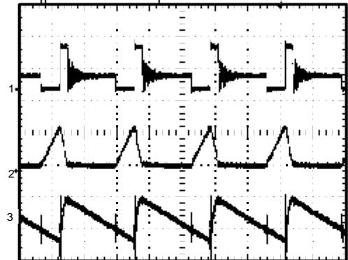
$V_{OUT} = 13.25V$ ,  $V_{IN} = 4.2V$  ; 8 LEDs
