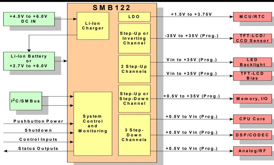
**Figure 1 – Applications block diagram featuring the SMB122 eight-channel, programmable DC/DC converter. This integrated power supply and battery manager provides precision regulation, monitoring, cascade sequencing, output margining and battery charging.**
