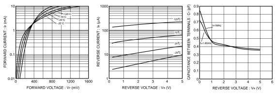
Fig.1 Forward characteristics
