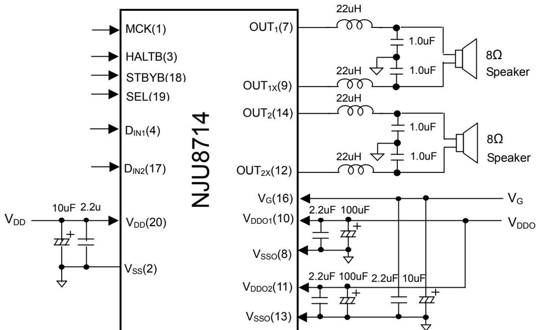
Note 3) De-coupling capacitors must be connected between each power supply pin and GND pin.
