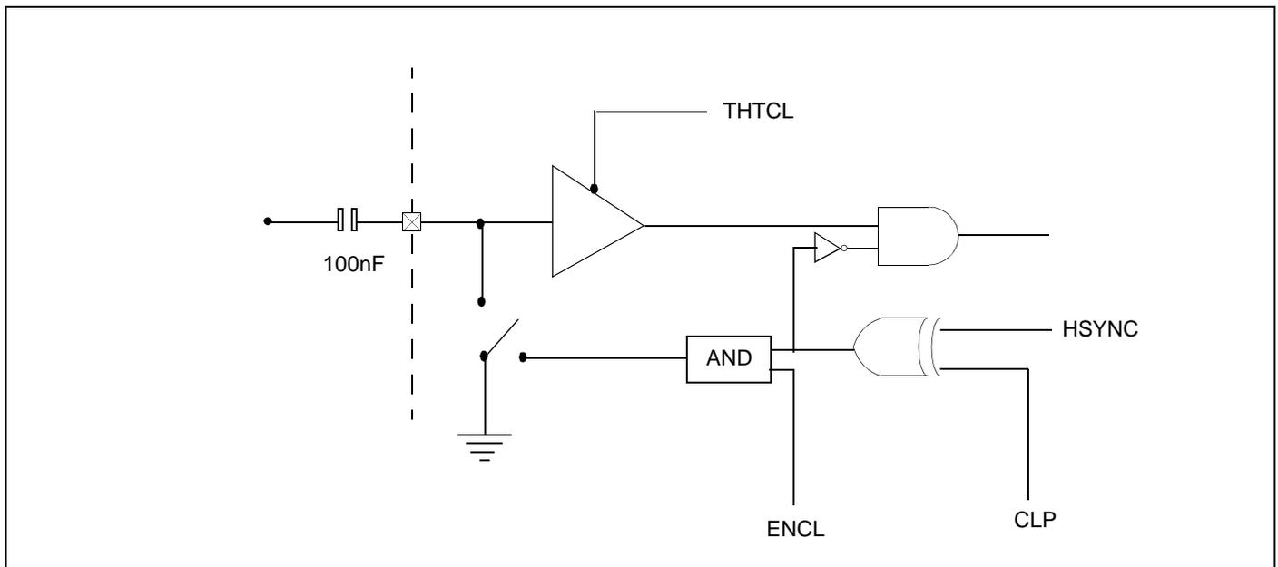
The input stage is configured by three control bits; THCTL, CLP and ENCL as shown in [Figure 37](#).
