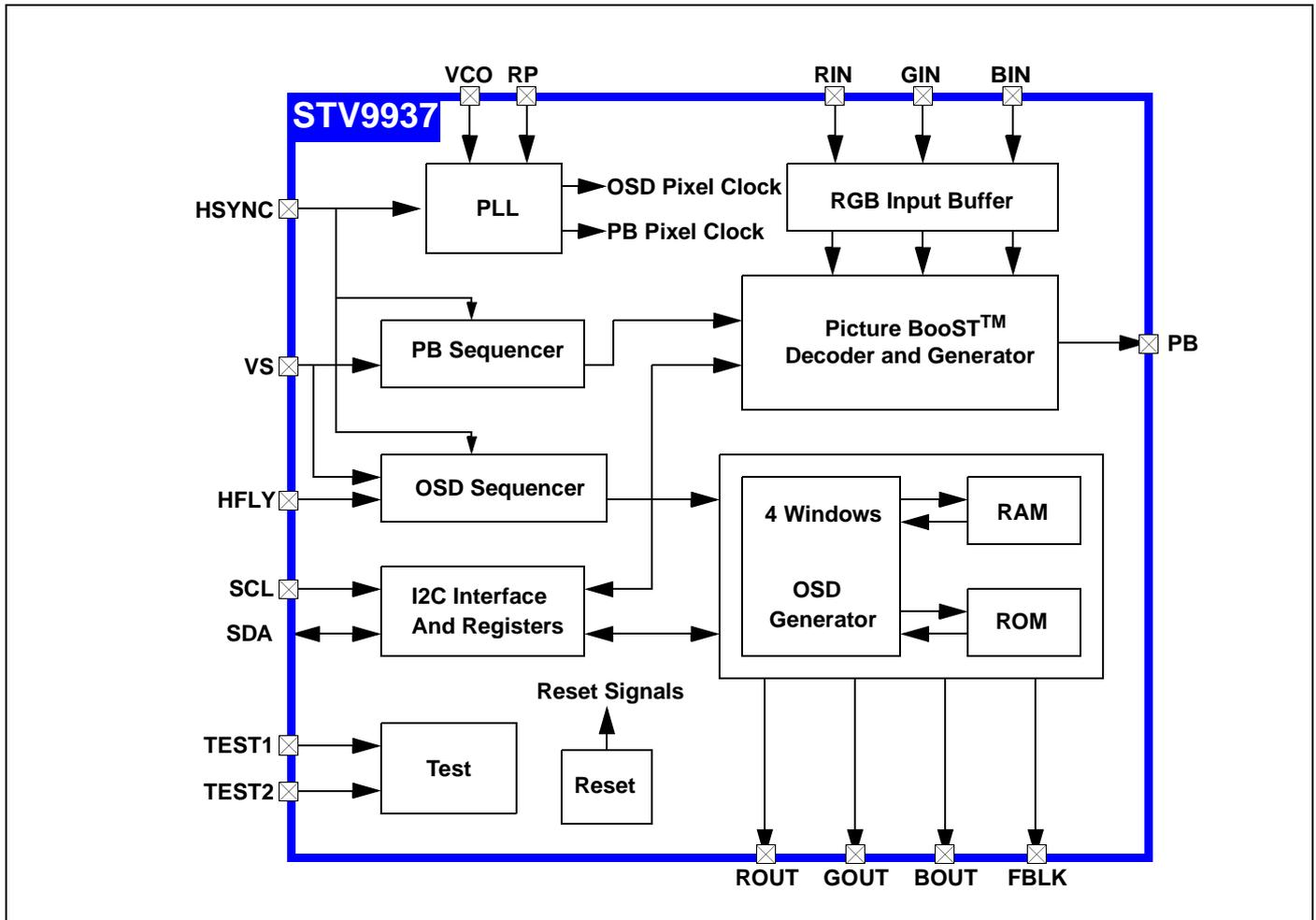
Figure 3: PictureBooST™ System Block Diagram
