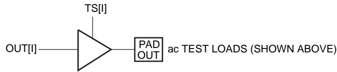
Figure 74. ac Test Loads
