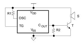
Note: a. R1 =1.2M $\Omega$  (S.R.=6KHz) , T (transistor) =  $\Omega$  > 150 ,S (speaker) =1/4W ,8 $\Omega$ ; all typical.
