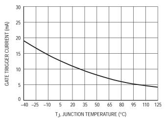
Figure 7. Typical Gate Trigger Current versus Junction Temperature
