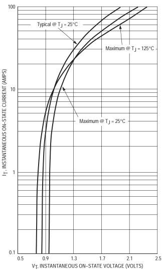
Figure 3. Typical On-State Characteristics
