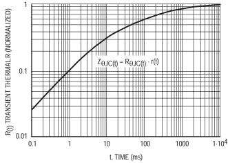
**Figure 4. Transient Thermal Response**
