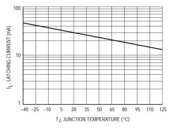
Figure 6. Typical Latching Current versus Junction Temperature
