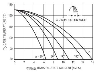
Figure 1. Typical RMS Current Derating
