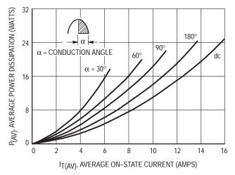
Figure 2. On State Power Dissipation
