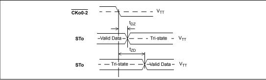
Figure 45 - Serial Output and External Control
