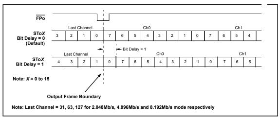
Figure 18 - Output Bit Delay Timing Diagram
