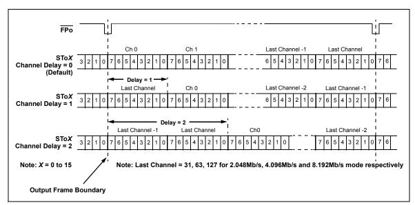
Figure 17 - Output Channel Delay Timing Diagram
