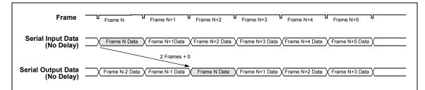
Figure 21 - Data Throughput Delay when input and output channel delay are disabled for Input Ch0 switched to Output Ch0
