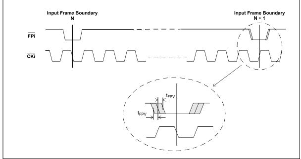
Figure 34 - Frame Boundary Timing with Input Frame Pulse (cycle-to-cycle) Variation
