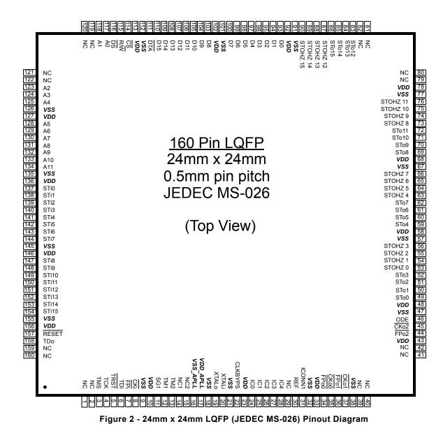
**PINOUT DIAGRAM:** (as viewed through top of package)
