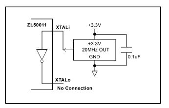
Figure 31 - External Clock Oscillator Circuit
