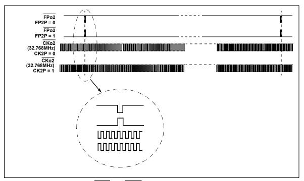
Figure 12 -  $\overline{PPO2}$  and  $\overline{CKO2}$  Output Timing when the CKFP2 bit = 0
