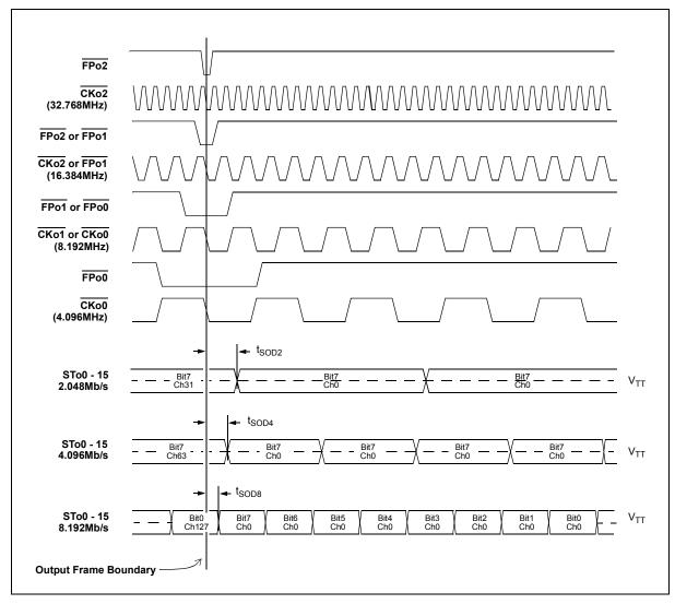
Figure 44 - ST-BUS Outputs (STo0 - 15) Timing Diagram
