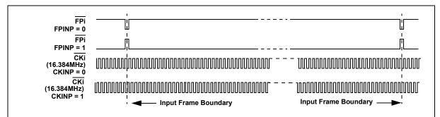
Figure 6 - Input Timing when (CKIN2 to CKIN0 bits = 000) in the control register
