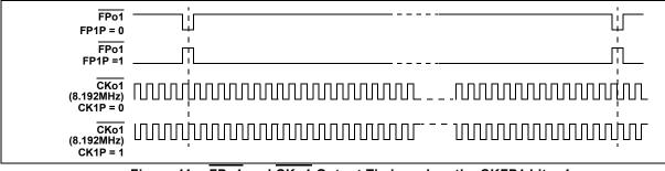
Figure 11 - FPo1 and CKo1 Output Timing when the CKFP1 bit = 1
