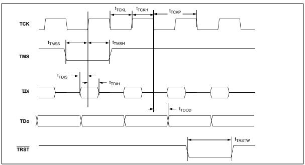
Figure 48 - JTAG Test Port Timing Diagram
