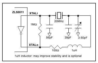
Figure 30 - Crystal Oscillator Circuit
