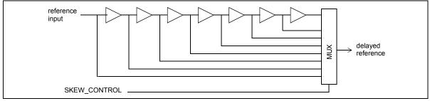
Figure 26 - Skew Control Circuit Diagram
