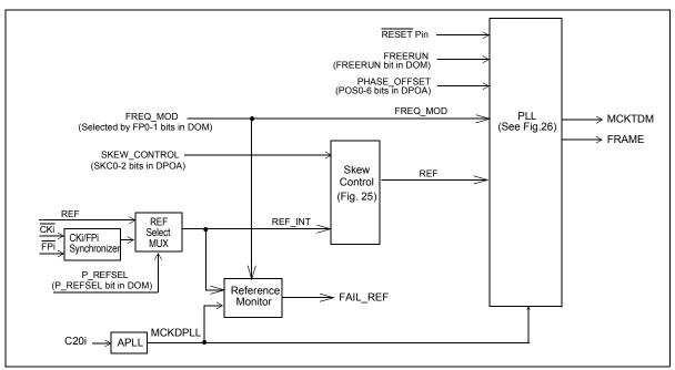
Figure 25 - DPLL Functional Block Diagram
