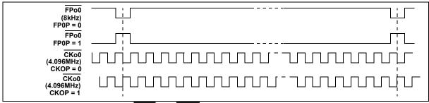
Figure 8 -  $\overline{FPo0}$  and  $\overline{CKo0}$  Output Timing when the CKFP0 bit = 0
