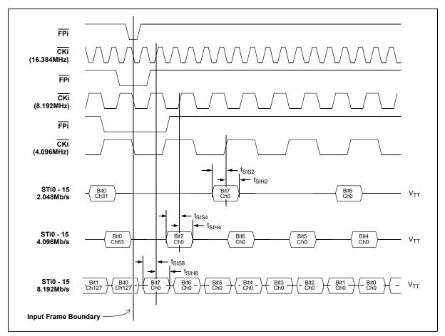
Figure 43 - ST-BUS Inputs (STi0 - 15) Timing Diagram
