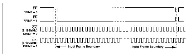
Figure 5 - Input Timing when (CKIN2 to CKIN0 bits = 001) in the control register
