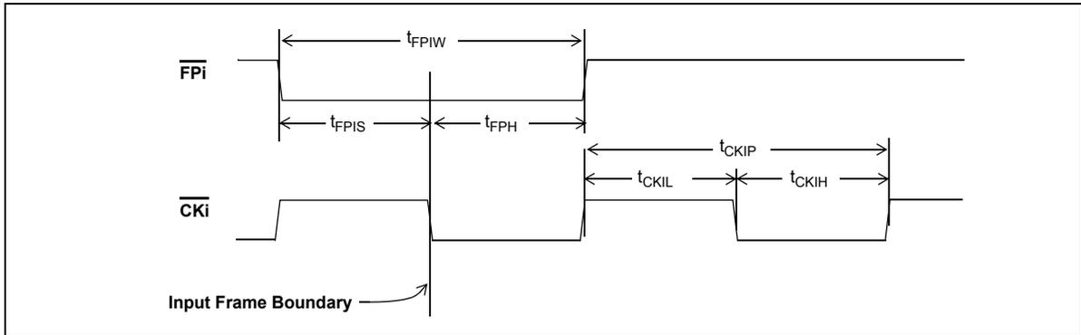
Figure 33 - Frame Pulse Input and Clock Input Timing Diagram
