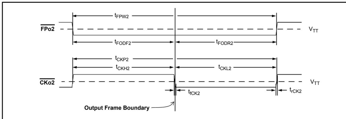
**Figure 43 -  $\overline{\text{FPo2}}$  and  $\overline{\text{CKo2}}$  Timing Diagram**
