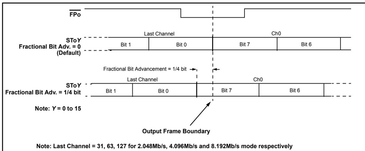
Figure 19 - Fractional Output Bit Advancement Timing Diagram
