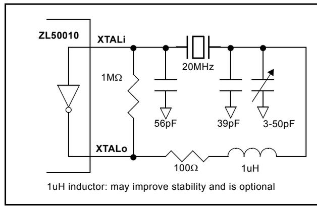
**Figure 31 - Crystal Oscillator Circuit**
