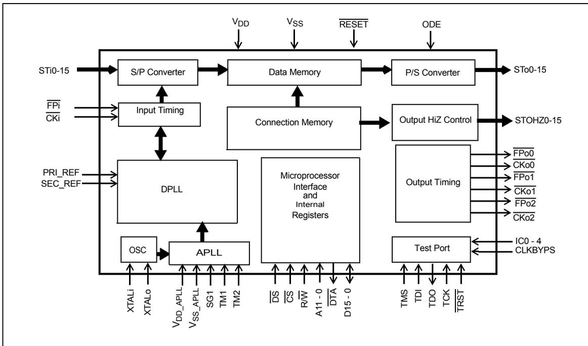
**Figure 1 - ZL50010 Functional Block Diagram**
