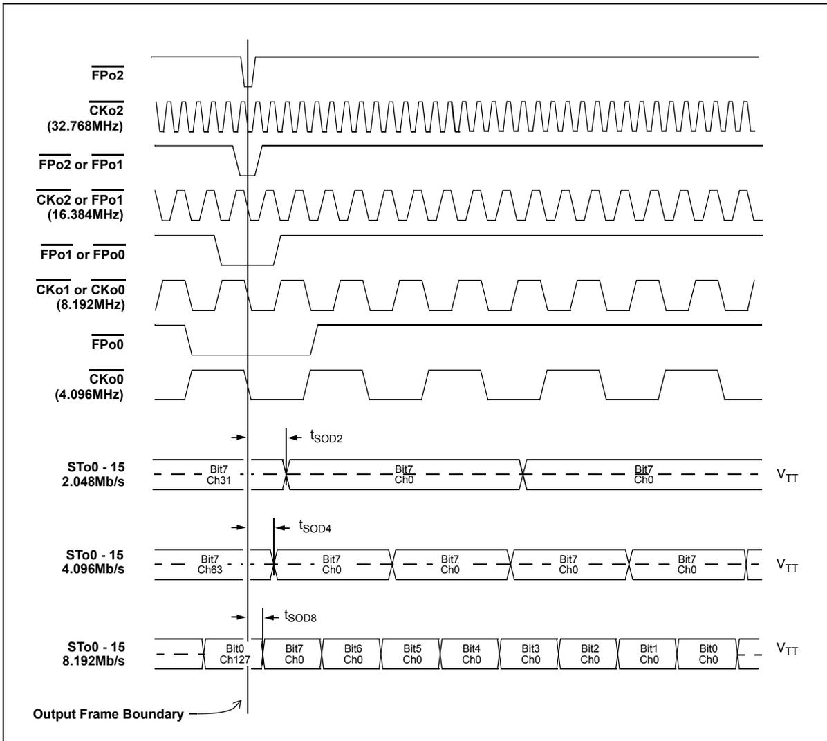
**Figure 45 - ST-BUS Outputs (STo0 - 15) Timing Diagram**
