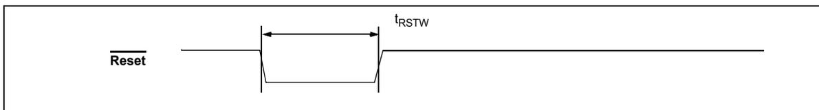
**Figure 50 -  $\overline{\text{Reset}}$  Pin Timing Diagram**
