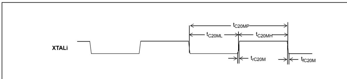
Figure 36 - XTALi Input Timing Diagram when Clock Oscillator is connected
