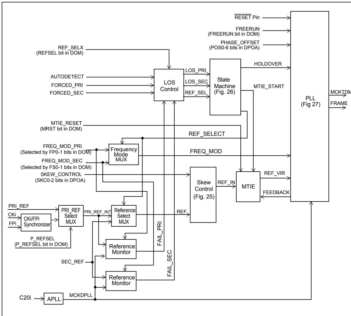
Figure 25 - DPLL Functional Block Diagram
