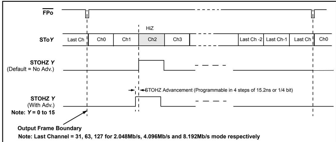
Figure 20 - Example: External High Impedance Control Timing
