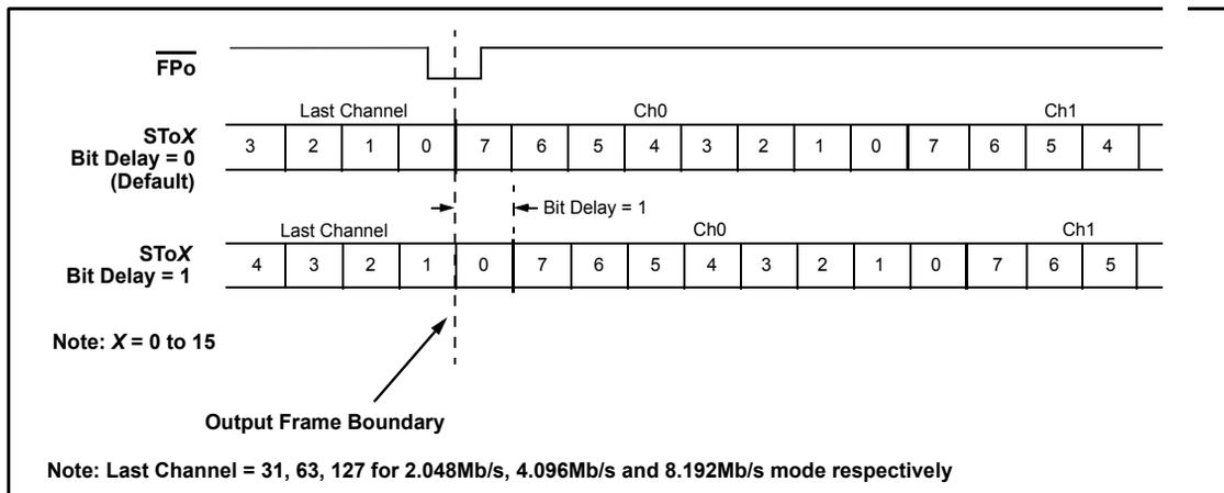
Figure 18 - Output Bit Delay Timing Diagram
