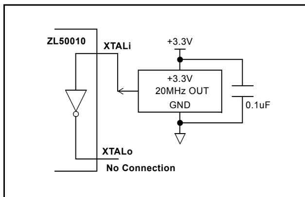
**Figure 32 - External Clock Oscillator Circuit**
