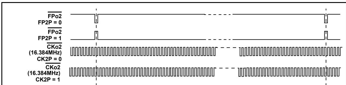
Figure 13 - FPo2 and CKo2 Output Timing when the CKFP2 bit = 1
