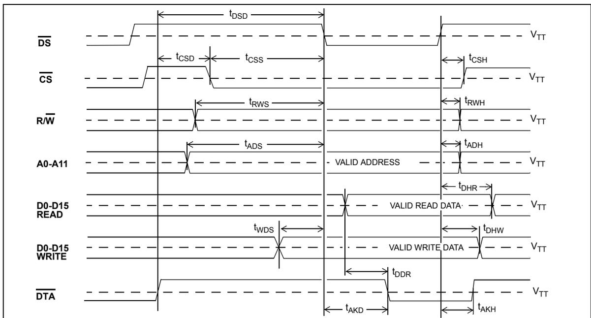
**Figure 48 - Motorola Non-Multiplexed Bus Timing**
