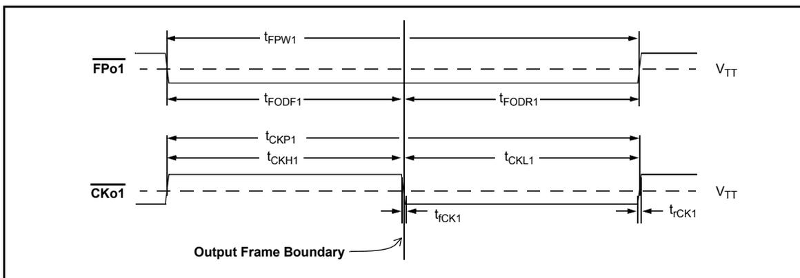
Figure 42 -  $\overline{\text{FPo1}}$  and  $\overline{\text{CKo1}}$  Timing Diagram
