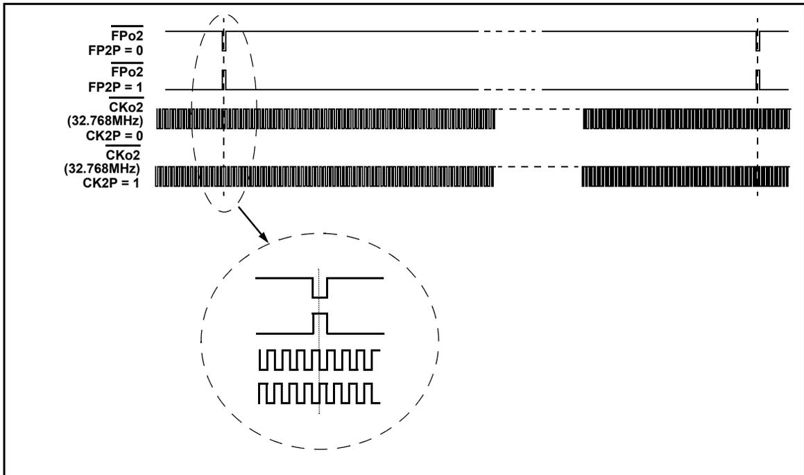
Figure 12 - FPo2 and CKo2 Output Timing when the CKFP2 bit = 0
