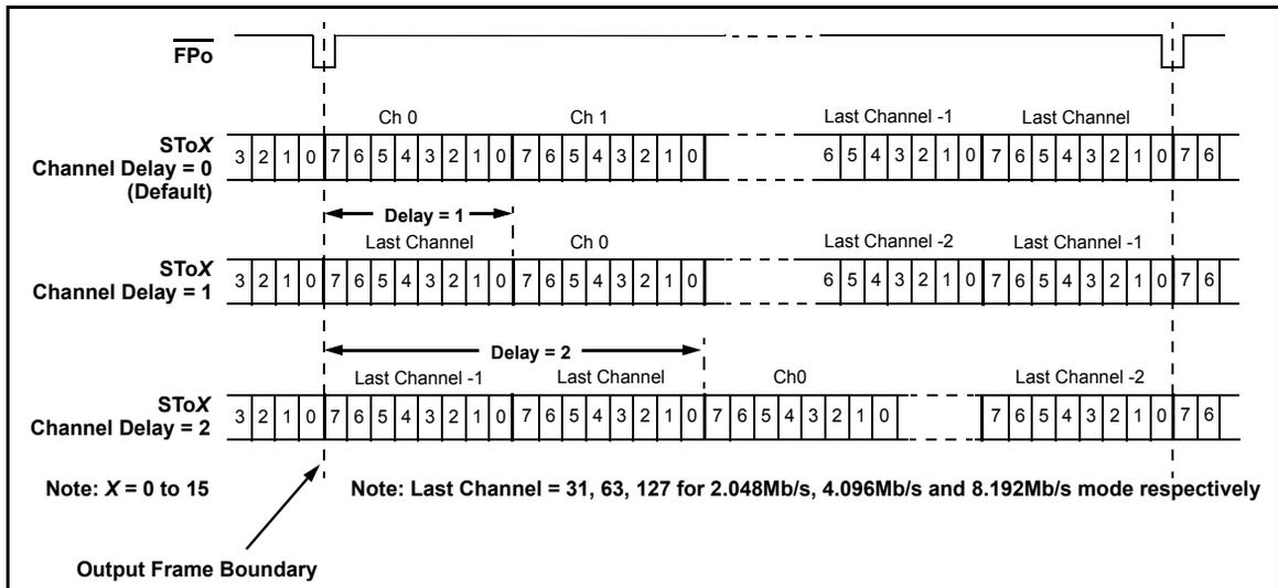
Figure 17 - Output Channel Delay Timing Diagram
