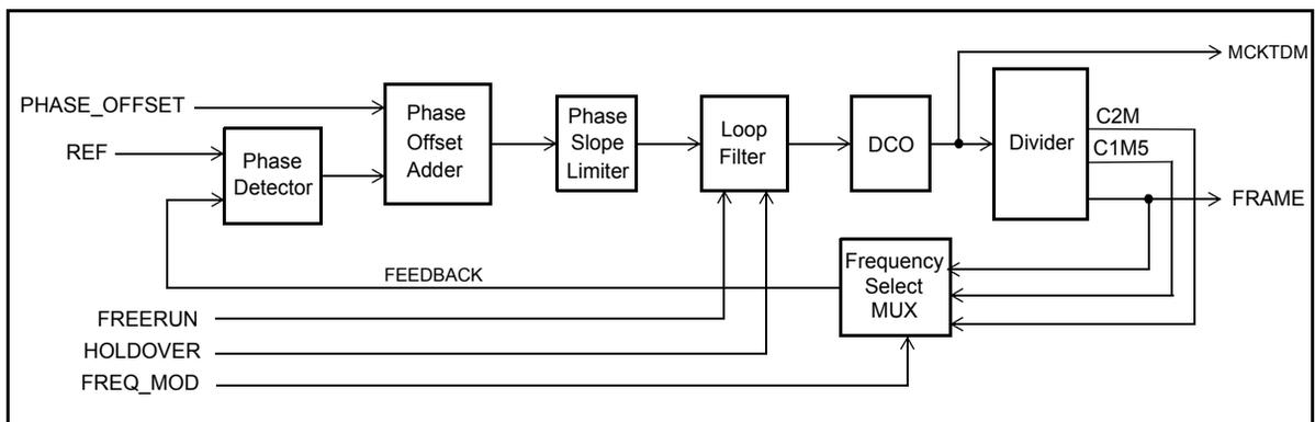
Figure 28 - Block Diagram of the PLL Module
