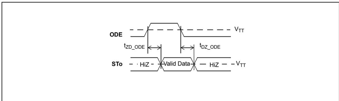
**Figure 47 - Output Driver Enable (ODE)**
