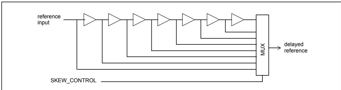
Figure 26 - Skew Control Circuit Diagram
