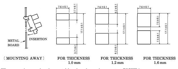
When mounting on other than metal board as shown above, contact TOSHIBA.
