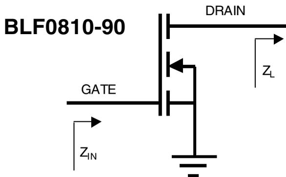
Fig.11 Definition of transistor impedance.
