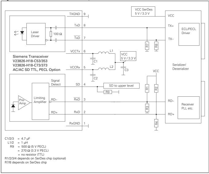
The power supply filtering is required for good EMI performance. Use short tracks from the inductor L1/L2 to the module  $V_{CC}Rx/V_{CC}Tx$ .
