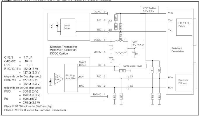
Values of R1/2/3/4 may vary as long as proper 50  $\Omega$  termination to V<sub>EE</sub> or 100  $\Omega$  differential is provided. The power supply filtering is required for good EMI performance. Use short tracks from the inductor L1/L2 to the module V<sub>CC</sub>Rx/V<sub>CC</sub>Tx.
