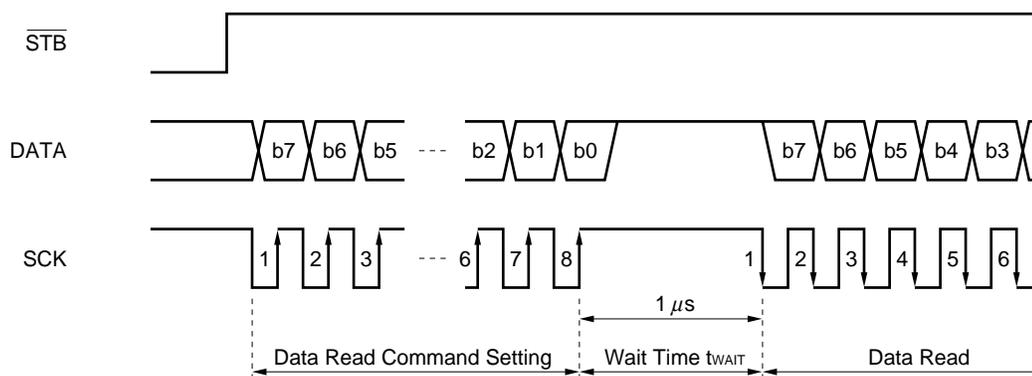
**Caution** As the DATA pin is an Nch open-drain output, a pull-up resistor must be connected externally (1 kΩ to 10 kΩ).
