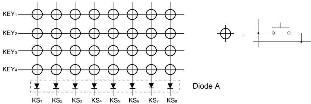
In this example, if 3 or more keys are simultaneously pressed, switches in the OFF state may be inadvertently judged as being ON.
