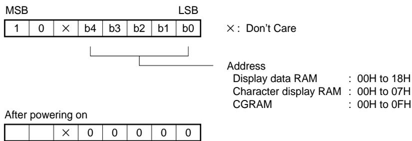
**Caution** If an unspecified address is set, data cannot be written until a correct address is next set. The address is not incremented even in increment mode.
