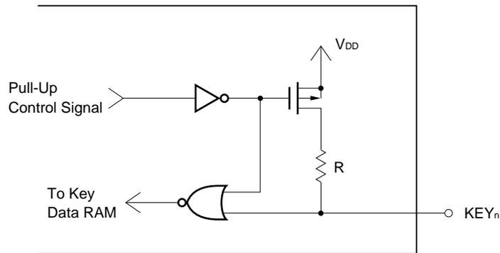
**Remark** In the event of key source output, the pull-up control signal becomes “H”, and the pull-up transistor is turned on.
