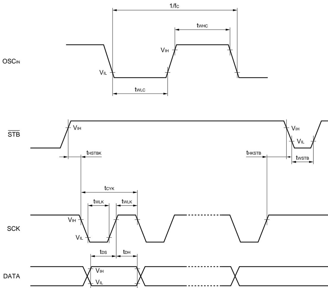
Switching Specification Waveform Diagrams (2/2)
