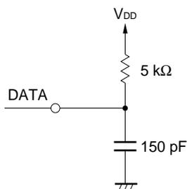
Switching Specifications Waveform Diagrams (1/2)
