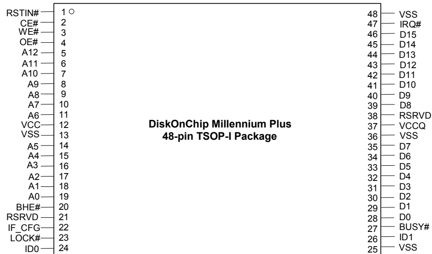
Figure 1: Standard Interface TSOP-I Pinout (Top View)
