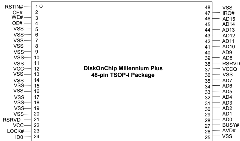
Figure 4: Multiplexed Interface TSOP-I Pinout (Top View)
